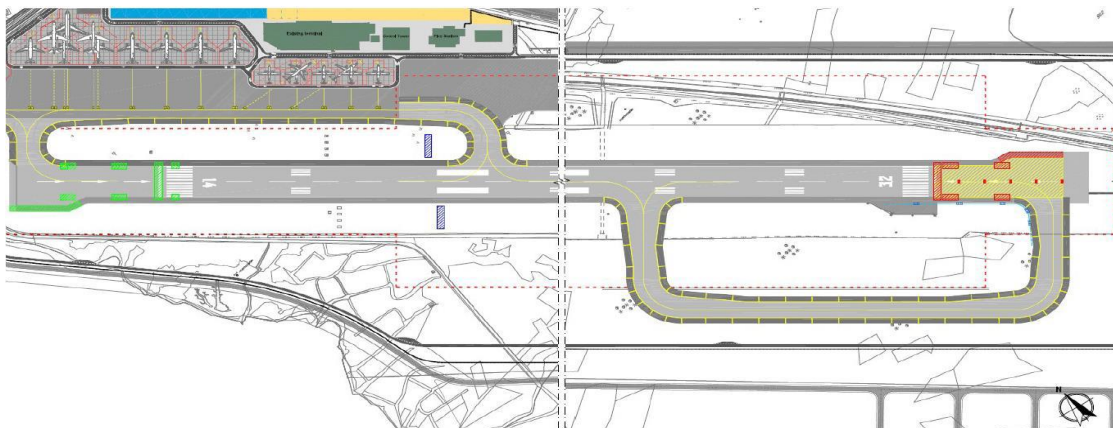
Figure 6-5: Component 3 - Runway 32 started extension and displacement of Runway 14 threshold
