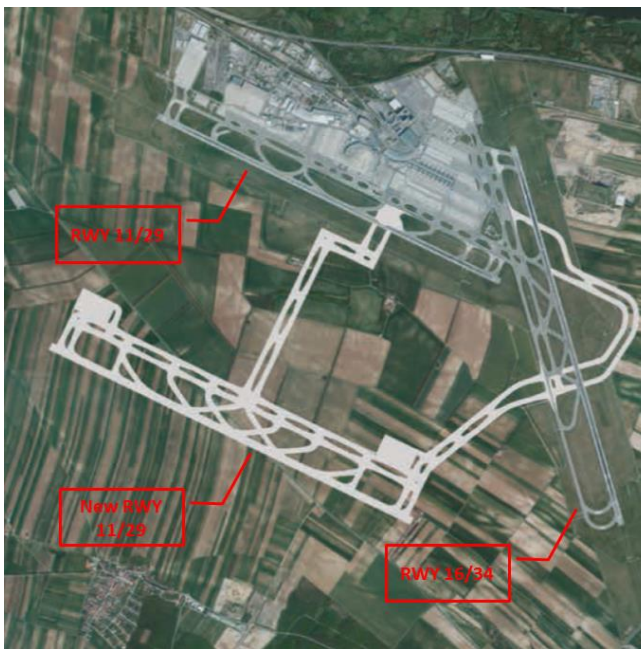
Figure 5-12: Localisation of the third runway of VIA
